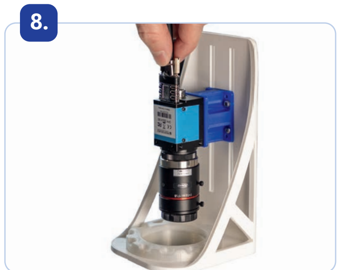
8. Attach the camera cable.
