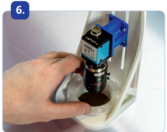
6. Attach the pre-assembled camera mount (step 4) to the LED panel using the cuff nut.
