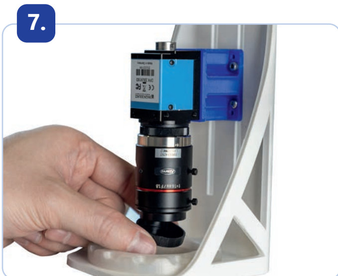
7. Remove the protective cap from the lens and then lower the camera.
